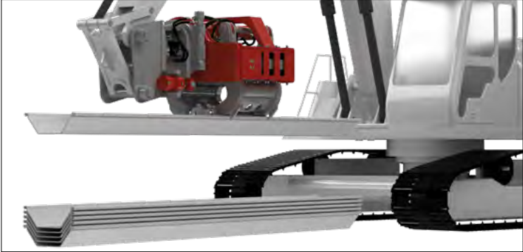
Carrying Sheet Piles
