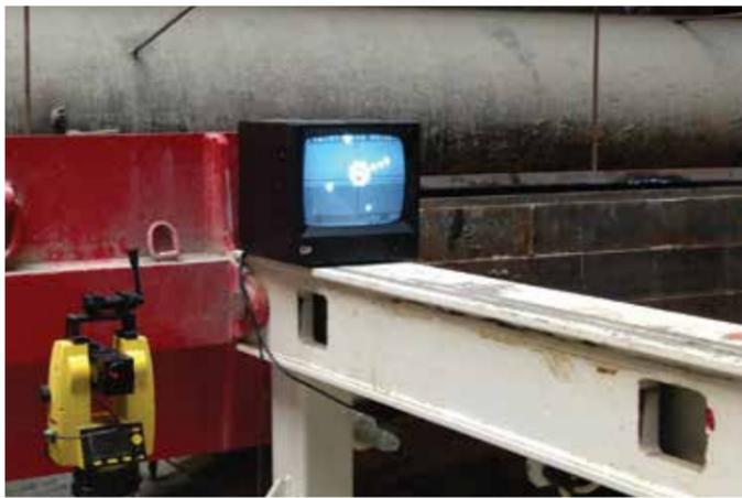
KBM Series can provide required slope and direction with high precision. This Camera Controlled Guided Boring System is used in the pilot drilling stage. A special system is inserted in the directional head, and the camera system follows the path from inside the drill stems.
